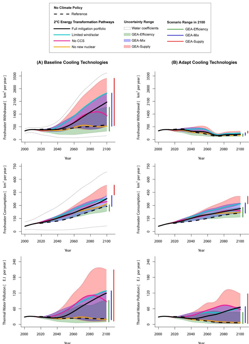
Figure 1: Global water impacts across the 2°C and reference scenarios for the two thermal power plant cooling technology cases: (A) baseline cooling technologies; and (B) adapt cooling technologies (transitioning away from once-through cooling)
